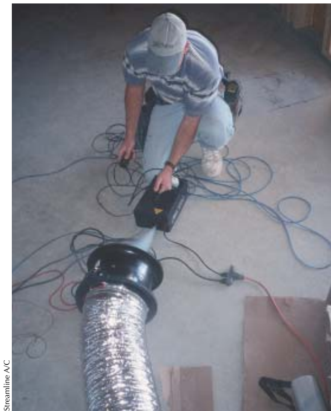
Figure 4. When a system exceeds the allowable air leakage standard, the author uses a theatrical fog generator to introduce visible vapor into the Duct Blaster fan intake. The fog makes it easy to find the leak locations.
