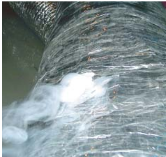
Figure 4. When a system exceeds the allowable air leakage standard, the author uses a theatrical fog generator to introduce visible vapor into the Duct Blaster fan intake. The fog makes it easy to find the leak locations.
