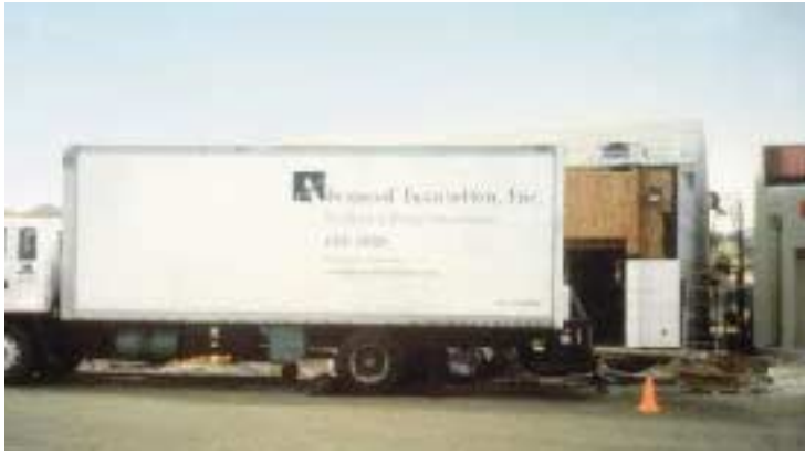
Figure 3. A 24-foot box truck holds up to 200 bags of insulation, as well as the blower, water supply, and other equipment. We try to get as close to the job as possible, but our equipment is powerful enough to push material up to 250 feet if necessary.
