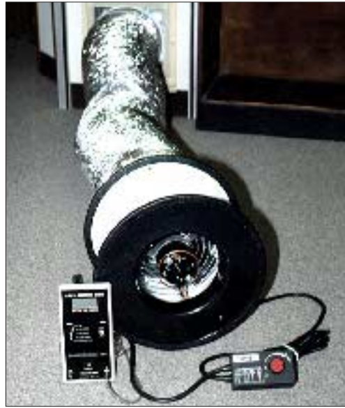
Figure 4. Measuring duct leakage takes under half an hour using the new Duct Blaster, a portable calibrated fan. Used as a powered flow hood, it can also accurately measure air flow through the duct system.
