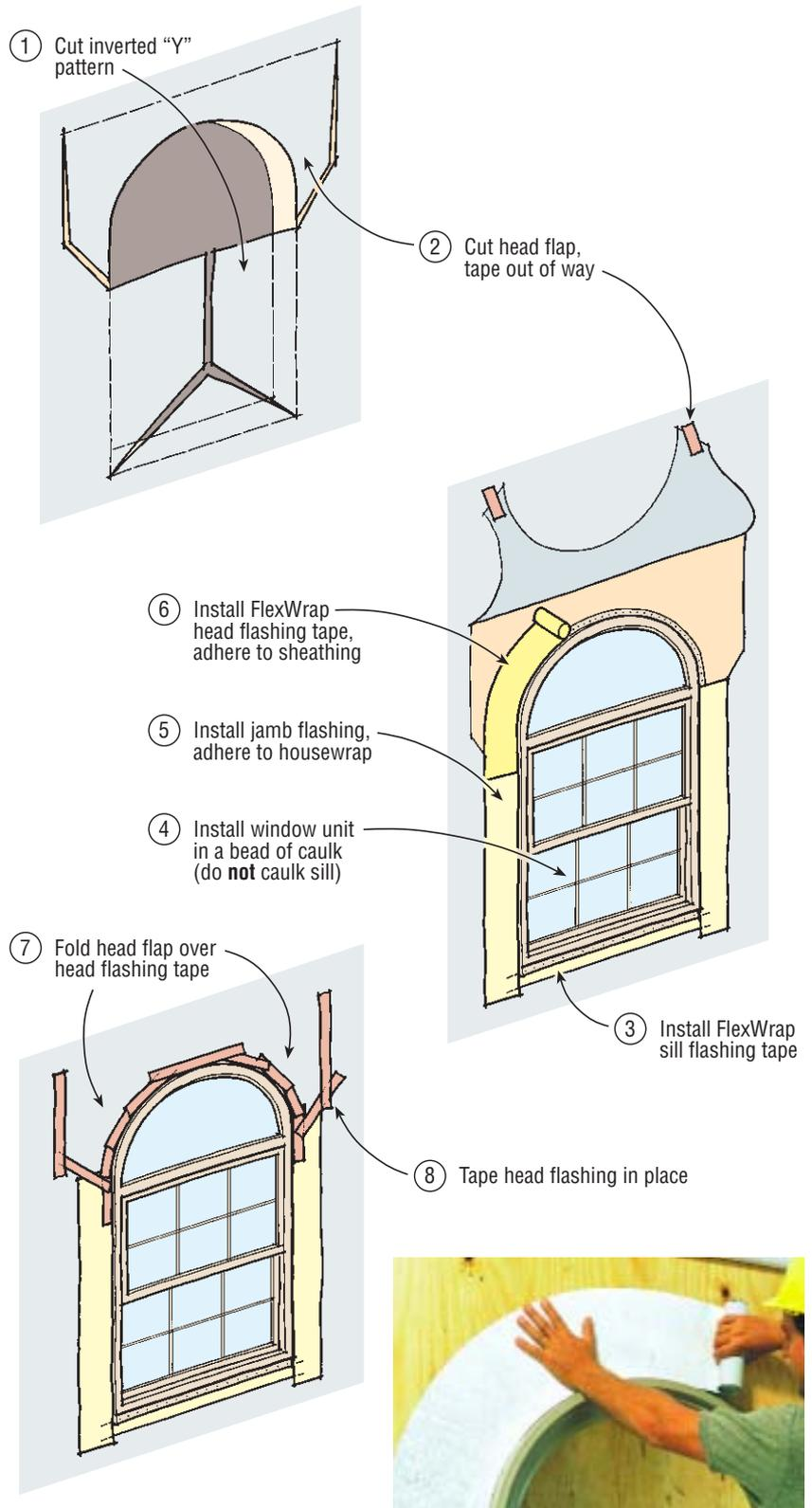
followed by the FlexWrap head flashing tape. To avoid a reverse lap, the head flashing should adhere directly to the sheathing, *not* the house wrap. The head flap is then folded over the head flashing tape and taped in place. A second piece of housewrap can be cut and inserted in a slit cut above the head flap. This second piece extends at least 12 inches beyond the head flap cut and is backup protection for the head flap taped seam.
